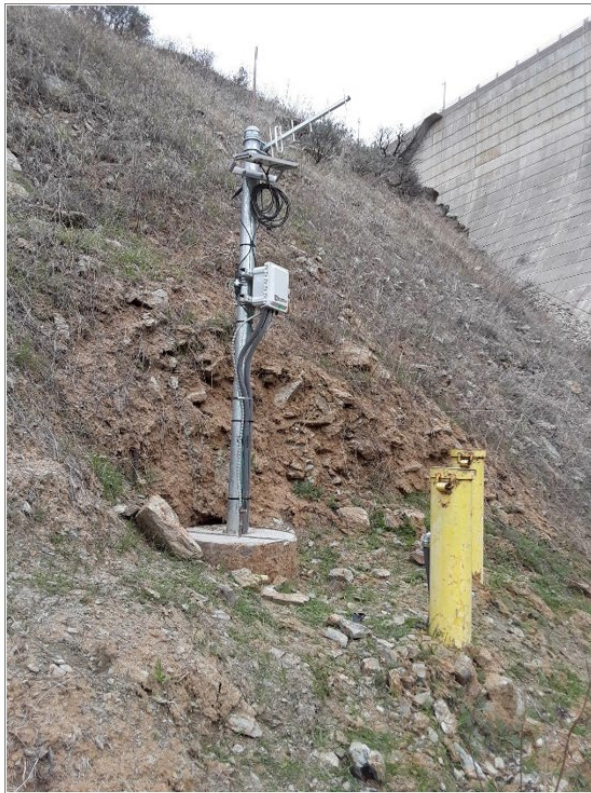
Figure 4-4. Dual Standpipe Piezometers
