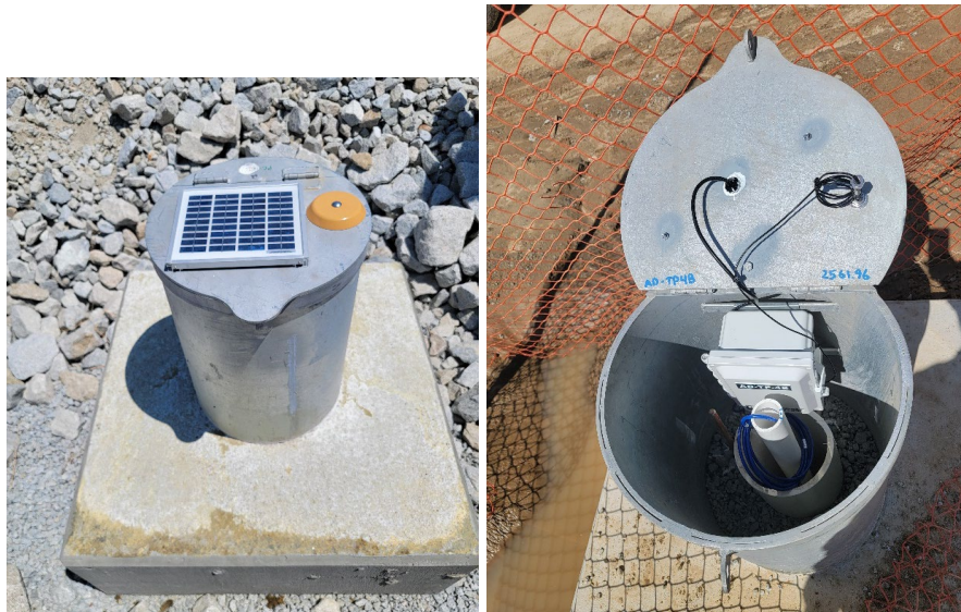
Figure 4-3. Typical Open-Standpipe Piezometer
