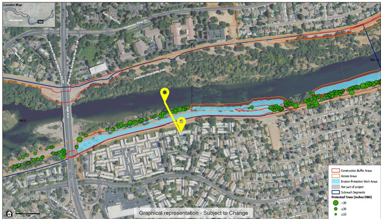
Figure 2-17. Layout of Segment 3-5 erosion protection feature and cross section location
