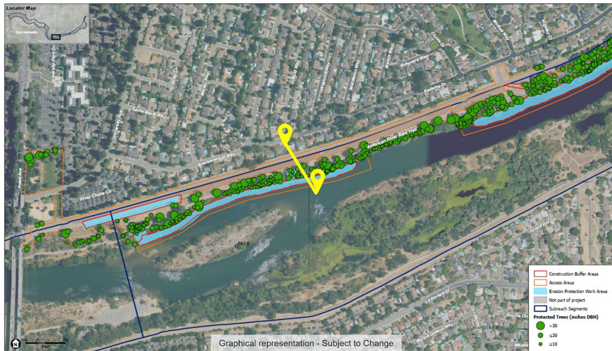
Figure 2-12. Layout of Segment 3-9 erosion protection features and cross section location
